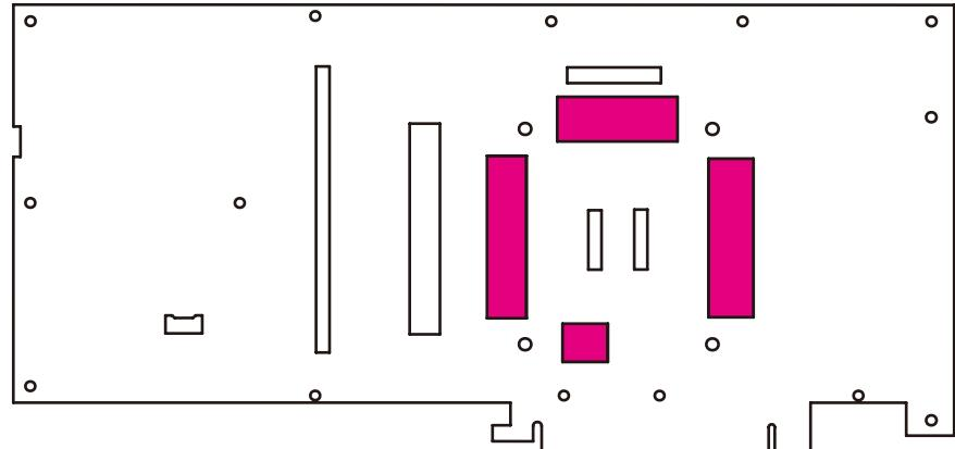
Thermal pad on correct positions.
