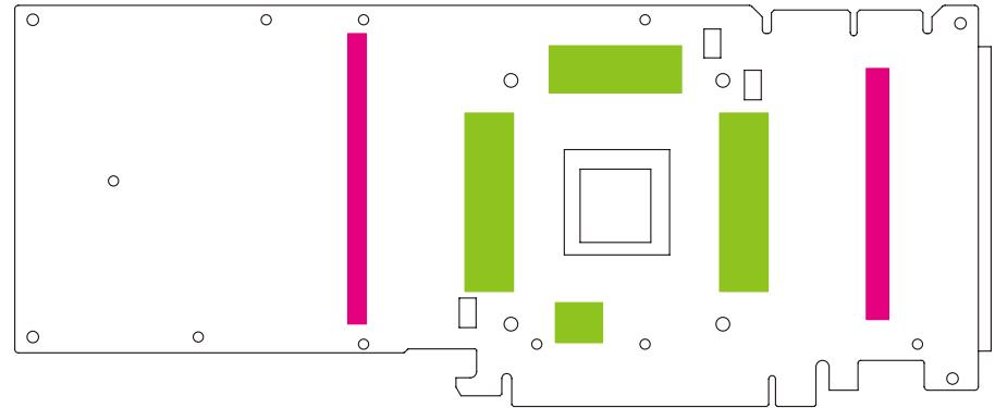
Applying the thermal pad and thermal paste on correct positions.
