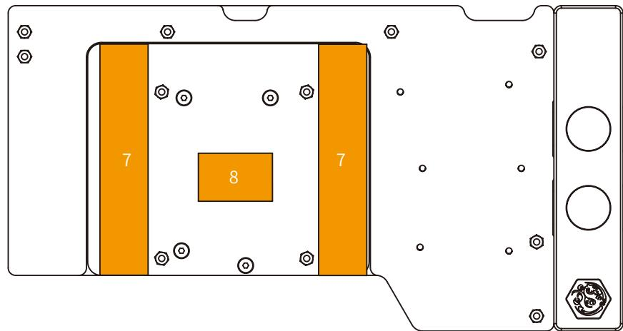
Make sure the correct thermal pads are in the appropriate locations.
