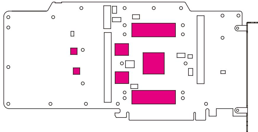
Thermal pad on correct positions.
