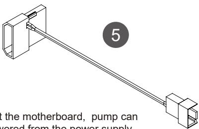
Except the motherboard, pump can be powered from the power supply via a patch cord.
