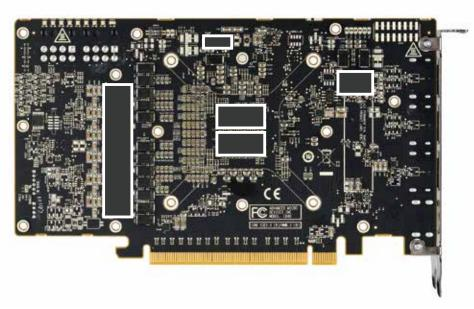
Applying The Thermal PAD And Thermal Paste On Correct Positions.
