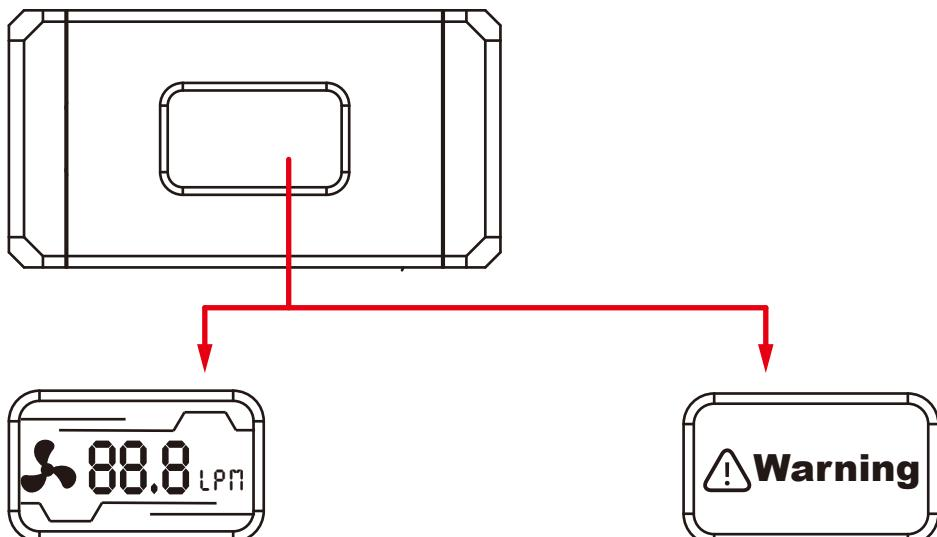
Product work interface, impeller with animation effect, The display flow range is 0.1~30.0LPM, fine Degree ±5%, when the flow rate is lower than 10.0LPM, The tens digit is not displayed.
