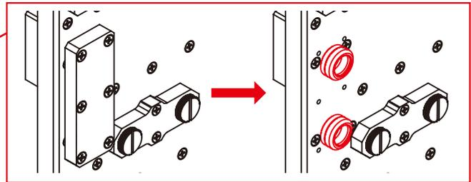
※ When installing the GPU, it is necessary to remove the conduit module, and then install the corresponding fittings.
