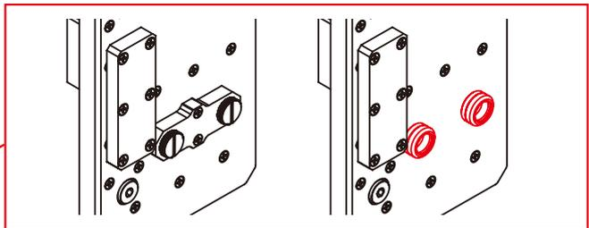
※ When installing the radiator, it is necessary to remove the conduit module, and then install the corresponding fittings.
