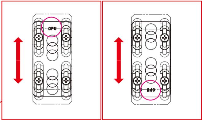
※ The position of the Hole position offset block can be adjusted to correspond to the CPU installation position of different motherboards.
