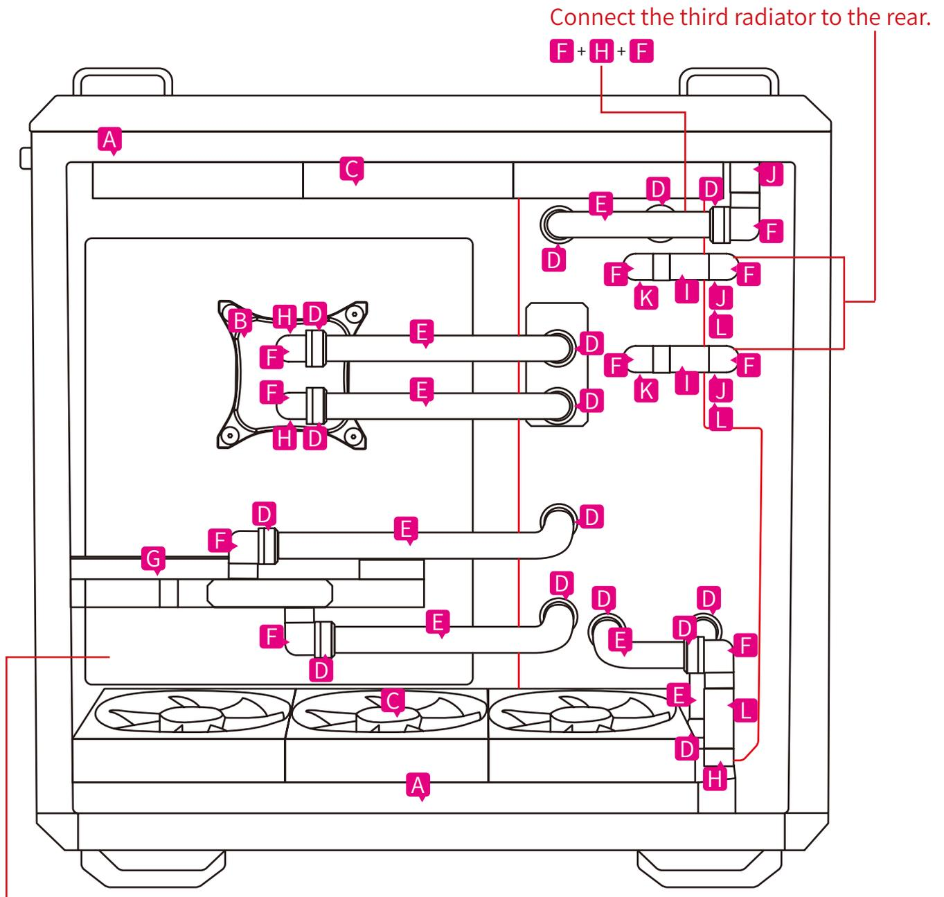
Three radiators installation methods, it is recommended to use m-ATX motherboard.
